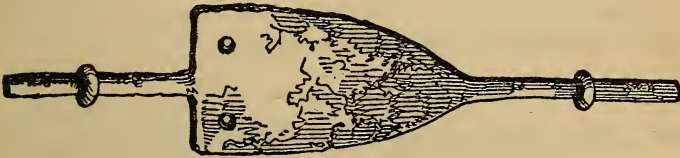
Bolt, showing holes for pricket wards of Key.
