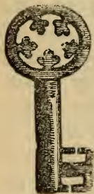
Piped Door-key with T shaped web or wards.
