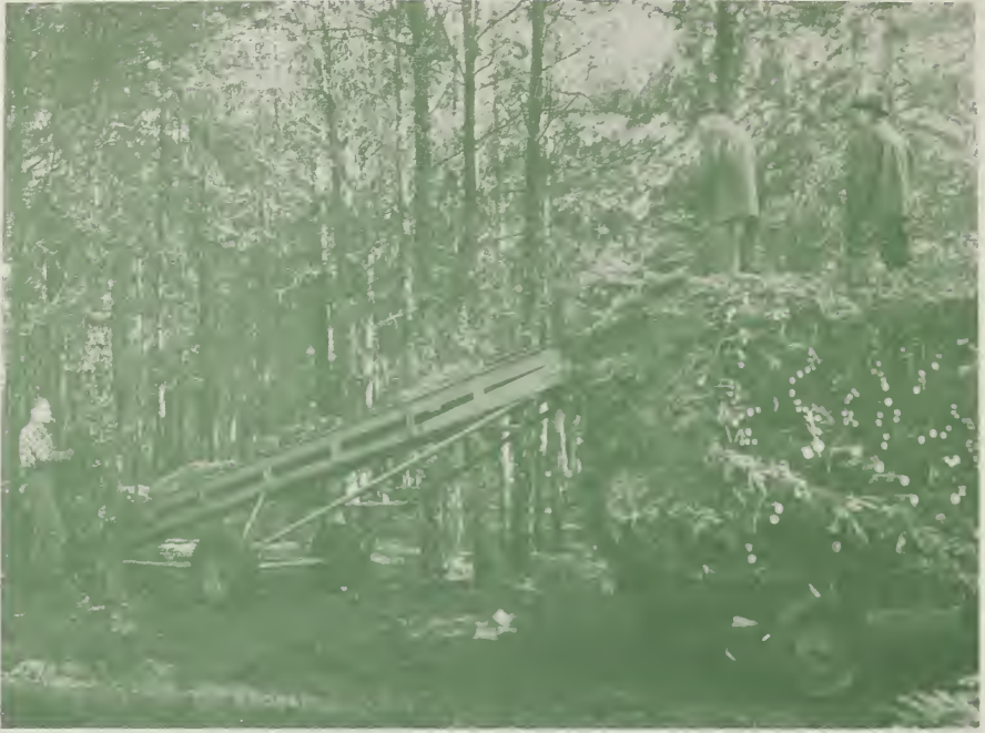
Loading baled Christmas trees on a truck trailer by means of a conveyor. State of Washington.
