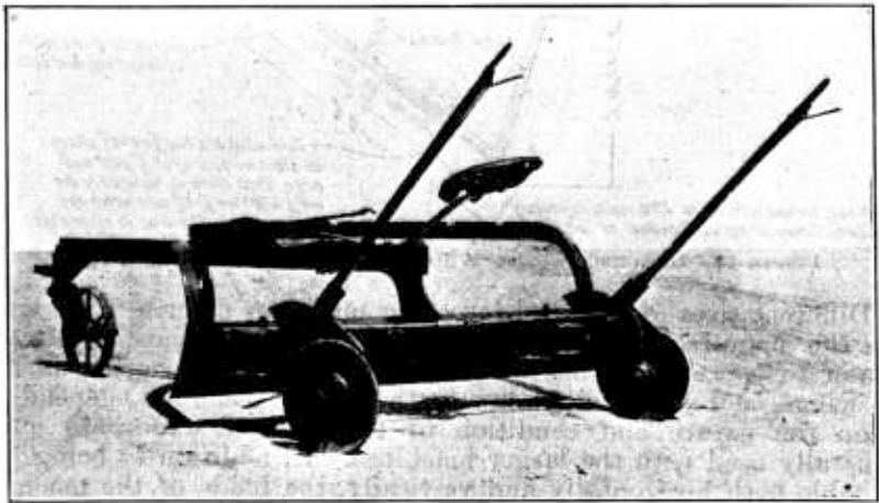
FIGURE 15.—A steel ditcher or terracer with steel revolving disks near each end of adjustable blade to hold blade in position
