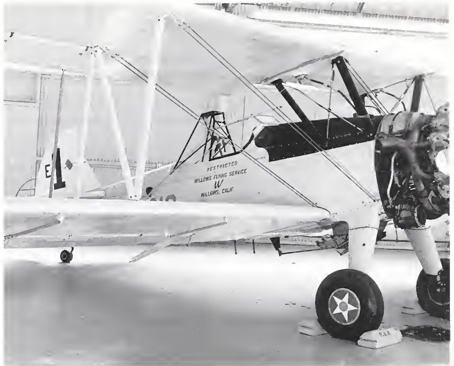
The Stearman NS Kaydet, modified for borate bombing, was used from 1934 into the 1940's as a training aircraft for basic training in the U.S. military. The first airtanker fleet, five Stearmans from Willows, CA, was organized for the Forest Service by Joseph Ely of the Mendocino National Forest and Willows Flying Service and used through equipment rental agreements with Willows.
