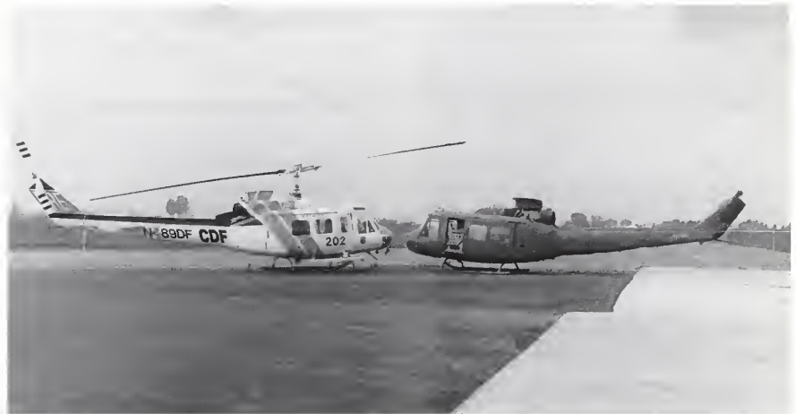
The EH-1H helicopter as obtained from the U.S. Army and Copter 202 CDF conversion.
