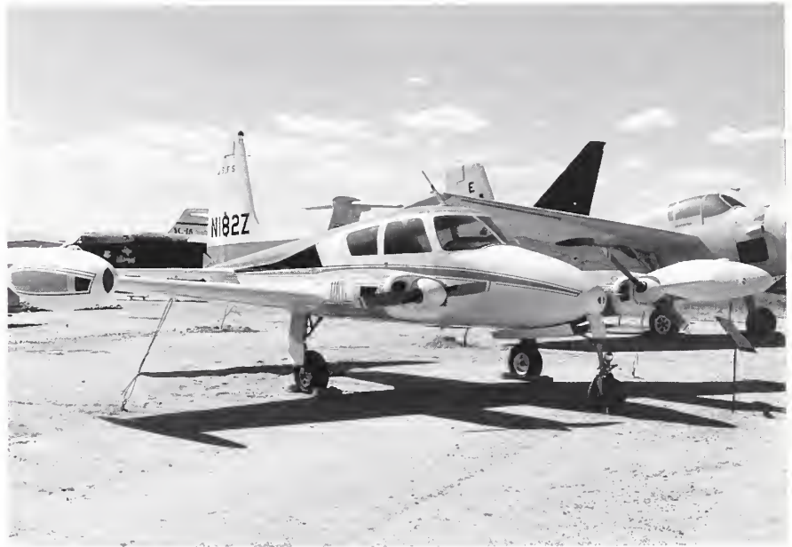
The Cessna 310 was the first twin-engine leadplane widely used by the Forest Service to lead and direct airtankers on retardant drops in 1968-69.
