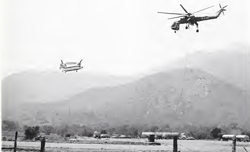
A Chinook B-234 with a 3,000-gallon (11,356-L) bucket (right) and a S-64 with a 2,000-gallon (7,571 L) bucket (left) filling up with fire retardant at the Mobile Retardant Base at the Stormy Fire Complex.
