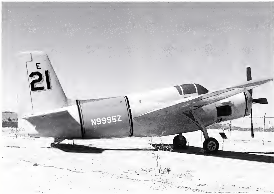
Tanker 21 is a Grumman AF-2S or "Guardian," a torpedo bomber modified for retardant bombing, operated by the Aero Union Corp. from 1950-57 on Forest Service and California Department of Forestry contracts.
