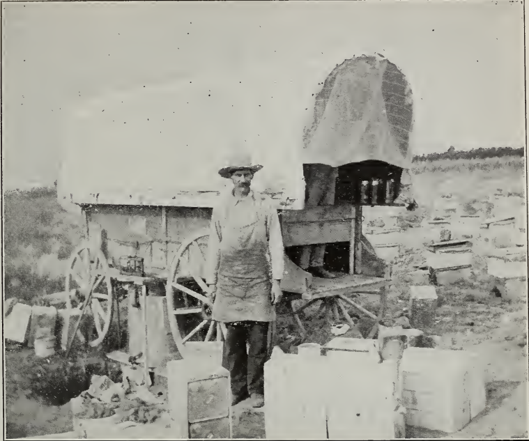
R. W. Ensley and his portable extracting-outfit having a capacity of 4400 lbs. of honey extracted and put in cans in 15 hours.
