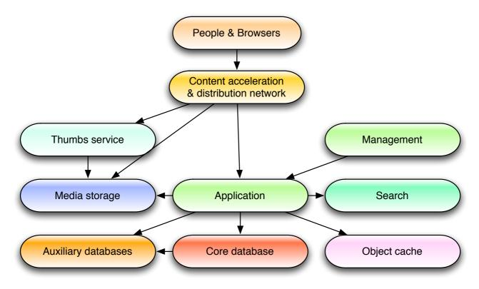
As application tends to be most resource hungry part of the system, every component is built to be semi-independent from it, so that less interference would happen between multiple tiers when a request is served.
