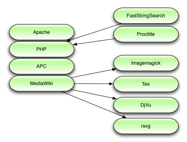
APC, the bytecode cache for PHP, should be treat as very important member of a stack, as running PHP applications without it (or alternatives) is a resource waste.
