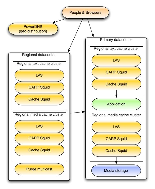
Content delivery network is the 'holy grail' of performance for Wikipedia. Most of pages (except for logged in users) end up generated in such a manner, where both caching and invalidating the content is fairly trivial.
