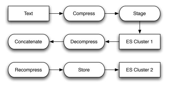
For external store extreme efficiency is achieved by recompressing - concatenating bunches of old revisions, then applying compression again. Efficient algorithms take similarity of revisions into account, ending up with 5%-10% of original size, instead of 30%-50% for single-pass compression.
