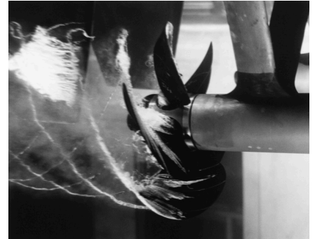
Cavitating propeller in water tunnel experiment
