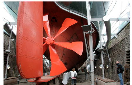
A replica of SS Great Britain 's first propeller was created for this museum ship. The real propeller was replaced with a four-bladed model in 1845. SS Great Britain was initially designed to have paddles but the design was modified after screw propellers were proven to be more effective and efficient.
