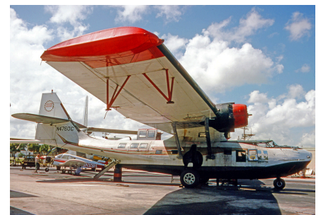
An OA-10A converted by Steward-Davis Inc to their Super Cat standard. It is additionally fitted out for survey work for Geoterrex Inc
