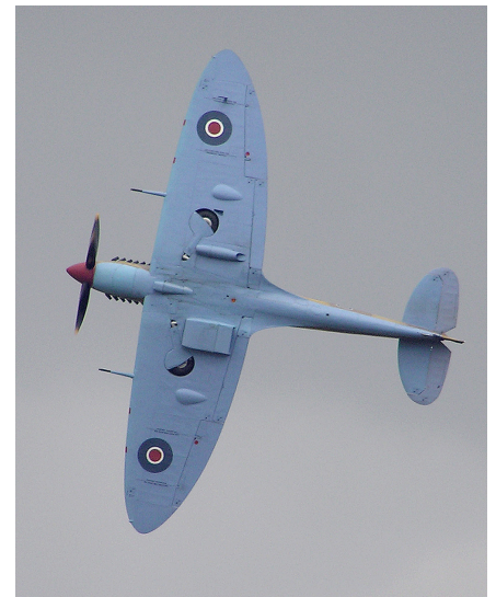
The Spitfire wing may be classified as: "a conventional low-wing cantilever monoplane with unswept elliptical wings of moderate aspect ratio and slight dihedral".
