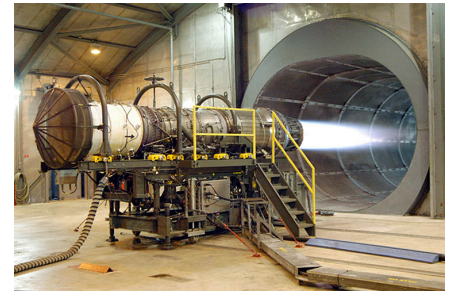
A Pratt & Whitney F100 jet engine is being tested. This engine generates thrust for a jet to propel it forward.
