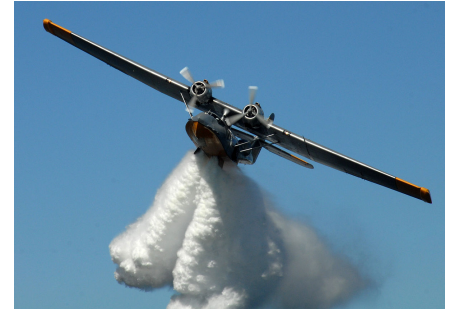
A PBY-6A Catalina drops a load of water from its bomb-bay doors
