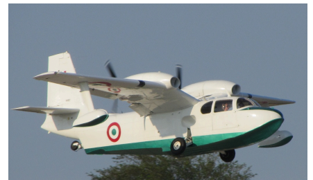
Italian Air Force Piaggio P.136 during takeoff retracting the wheels that make it an amphibian.
