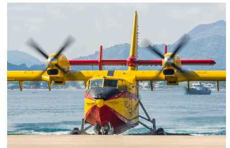
A Canadair CL-215T amphibian with retractable wheels
