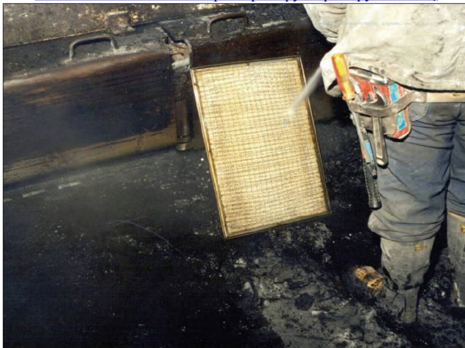
Figure 4-7.—Cleaning scrubber filter panel with water spray.
