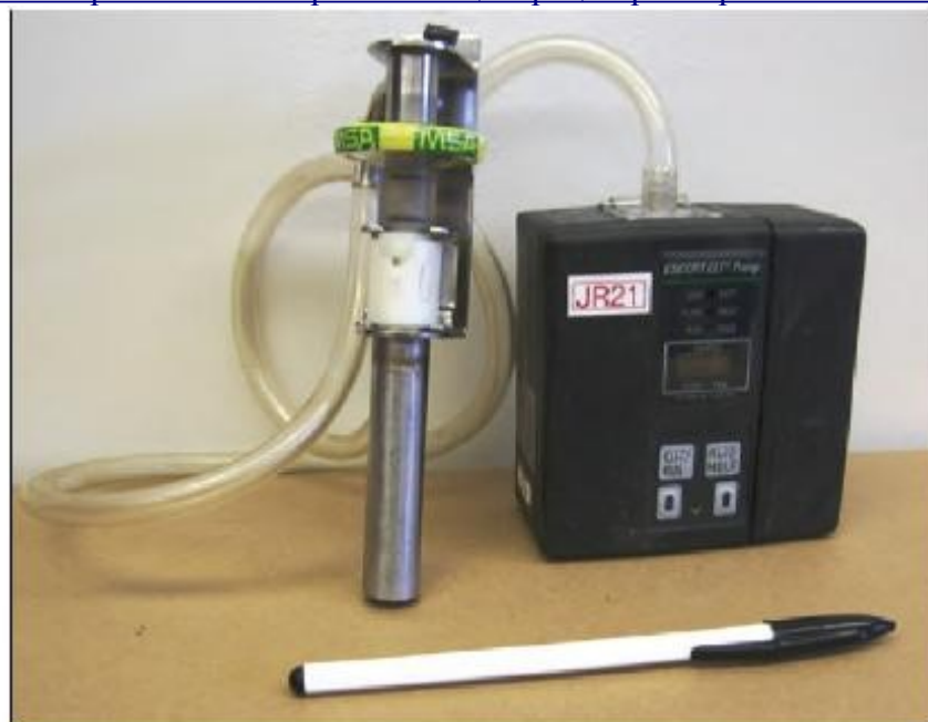
Figure 2-1.—Gravimetric sampling pump, cyclone, and filter cassette.
