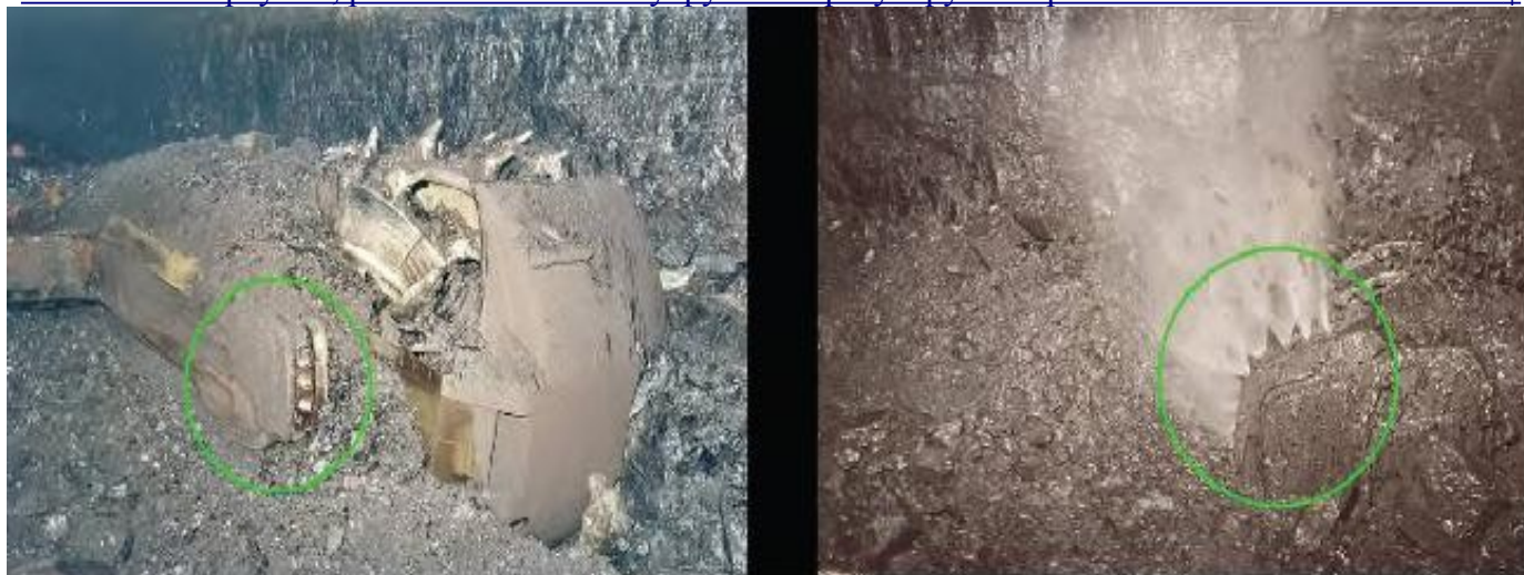
Figure 3-13.—Crescent sprays located on shearer ranging arm.
