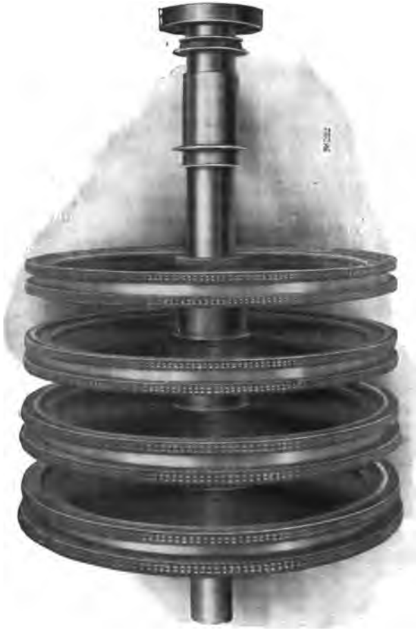
FIG. 117. Wheels and Shaft of a Four-stage Curtis Turbine.
