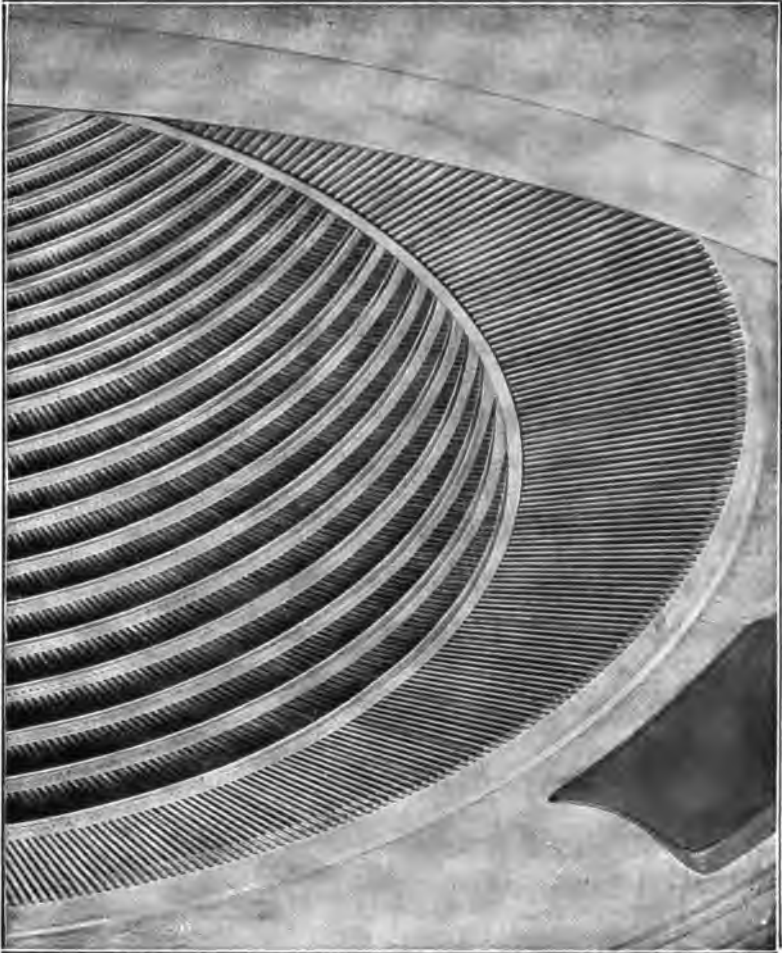
FIG. 99. Interior of an Allis-Chalmers Turbine Casing, Showing Blades Protected by Shroud Rings.
