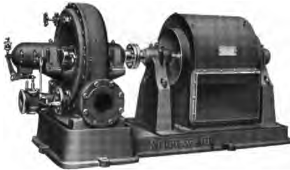
FIG. 148. Sturtevant Turbine Direct-connected to a Blower.
