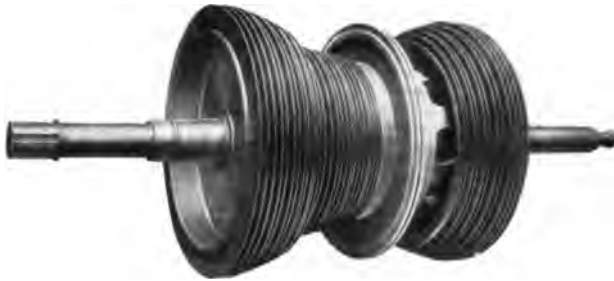
FIG. 109. Rotor of a Westinghouse Double-Flow Turbine.
