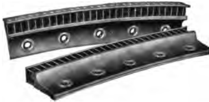
FIG. 115. Curtis Moving Blade Segments.
