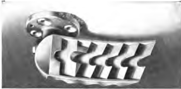
FIG. 144. Sturtevant Nozzle and Stationary Buckets, showing Flanged Connection to the Steam Chest.
