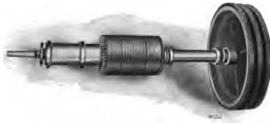
FIG. 125. Wheel, Shaft, Armature, and Commutator of a Small Curtis Turbine.
