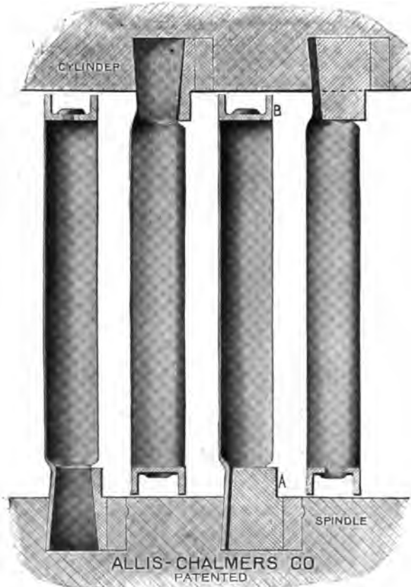
FIG. 97. Sankey's Blading for Parsons Turbines.
