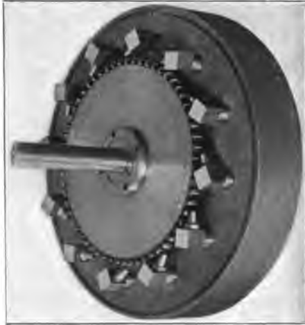
FIG. 149. Kerr Bucket Wheel and Nozzles.
