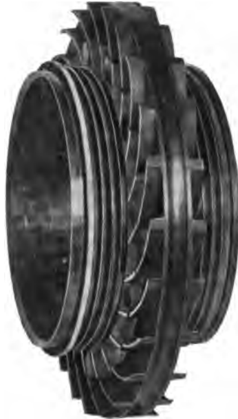
FIG. 93. Propeller of a Water-packed Gland of a Westinghouse-Parsons Turbine.
