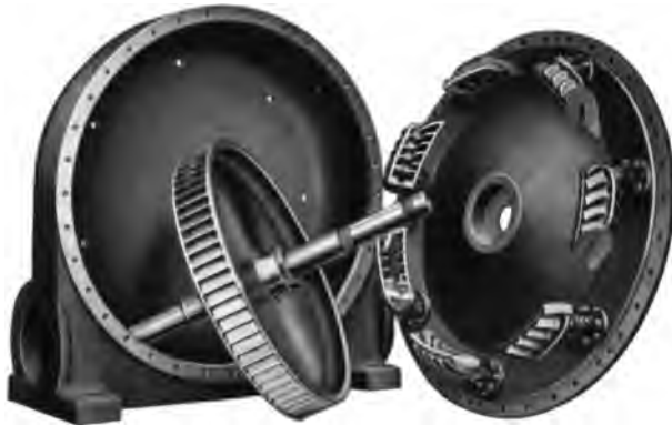
FIG. 143. Sturtevant Turbine with the Wheel Removed to the Side to Show the Arrangement of the Buckets.
