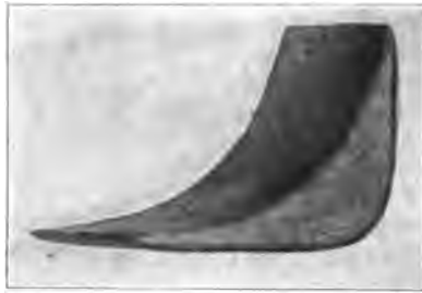
FIG. 58. Etched Section of a Blade made of Monnot Metal (Steel and Copper).
