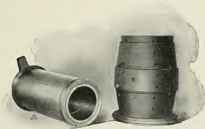
FIG. 99 —Bearing, with concentric brass sleeves, Westinghouse-Parsons turbine.
