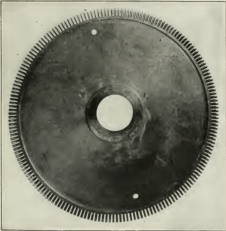
FIG. 115.—Buckets on one of the wheels of a 500-K.W. Curtis turbine.
