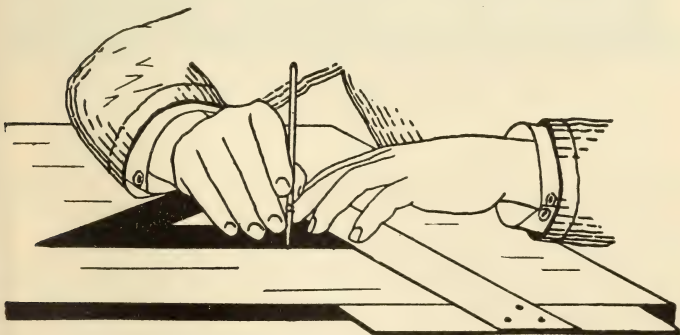
Fig. 10—Correct Manner of Holding a Ruling Pen.
