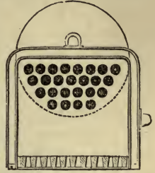
"BOILER OF ROCKET." 1829.
