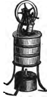
FIG. 2. Toy Engine with Oscillating Cylinder.
