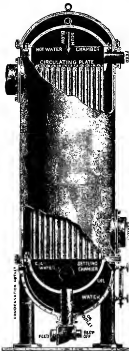
FIG. 56.—The Riblet Steam-feed Water Heater. The Water passes through the Tubes and the Steam on the outside.
