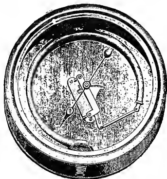
FIG. 47.—The Steam Gauge shown in Fig. 46, with Dial removed, showing the Tube upon which the Steam acts and the Gearing giving motion to the Pointer.
