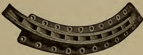
Fig. 86. Group of Nozzles for High-Pressure End
