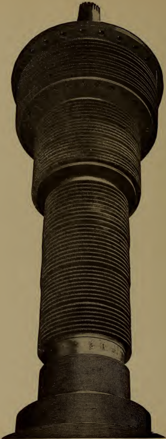
Fig. 103. Rotor of Westinghouse-Parsons Turbine with Balance Pistons
