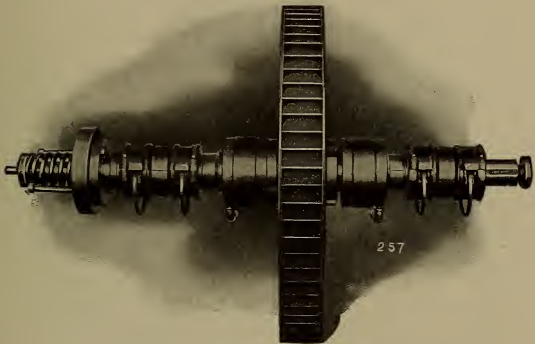
Fig. 48. Rotor and Shaft of Terry Single-Stage Turbine Courtesy of Terry Steam Turbine Company, Hartford, Connecticut
