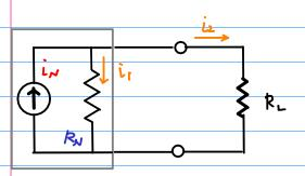
$$i_{l} = \frac{R_{L}}{R_{N} + R_{L}} i_{N}$$
