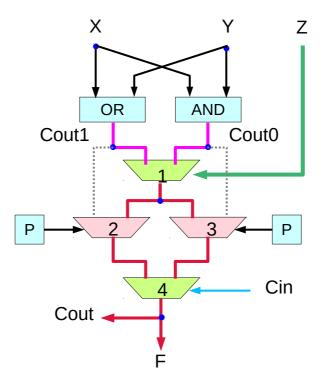
For the <u>first</u> cell in a carry chain with a <u>carry input</u> (provided by input Z), <u>mux2</u> and <u>mux3</u> both pass the value from <u>mux1</u>
