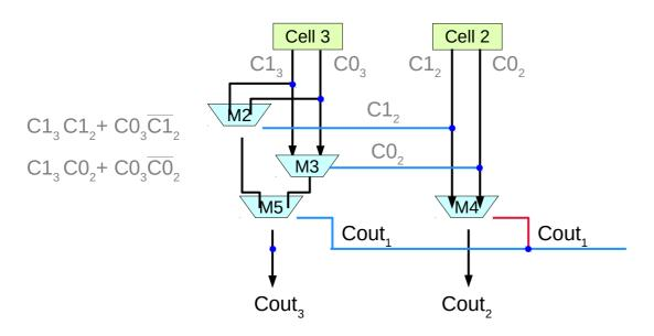
$$(C1_3C1_2 + C0_3\overline{C1}_2)Cout_1 + (C1_3C0_2 + C0_3\overline{C0}_2)\overline{Cout}_1$$
