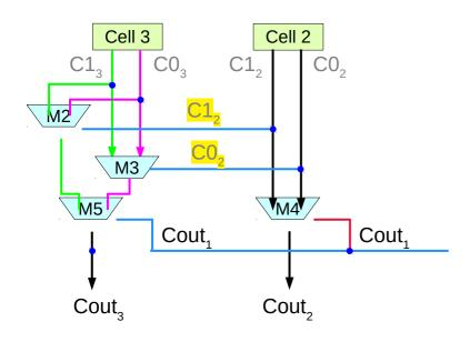
$$(C1_3C1_2 + C0_3\overline{C1}_2)Cout_1 + (C1_3C0_2 + C0_3\overline{C0}_2)\overline{Cout}_1$$
