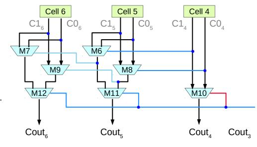
A Carry Select carry chain structure for use in FPGAs
