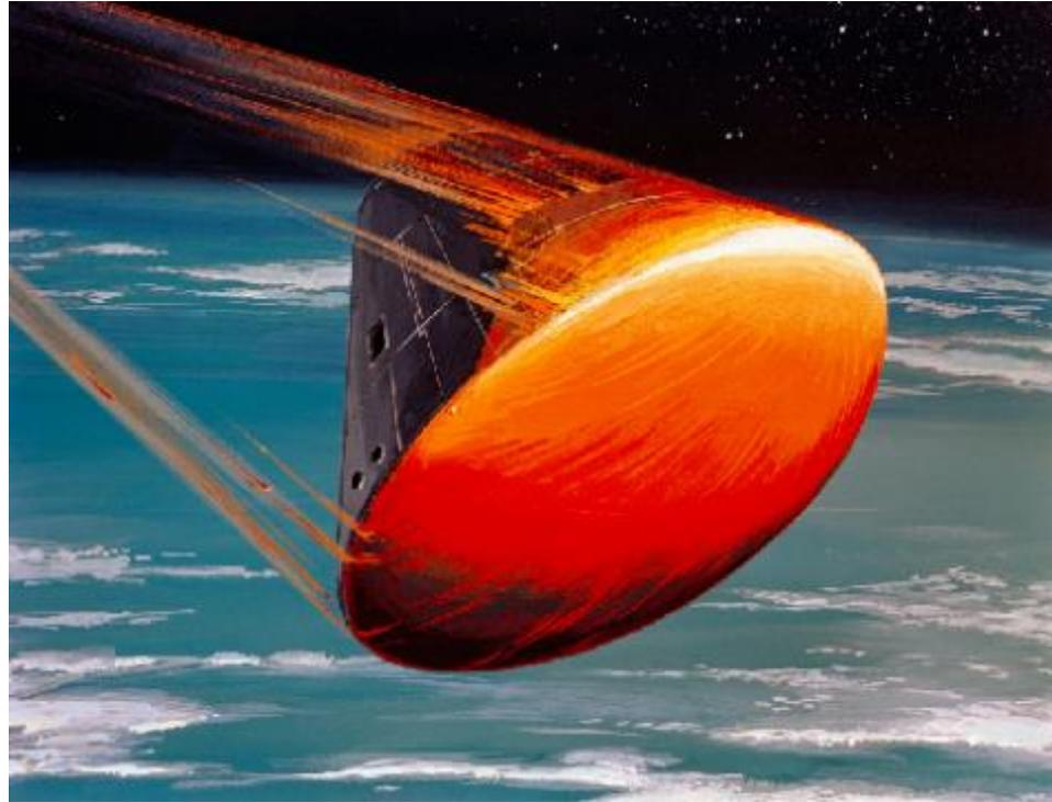
**Friction in Earth's Atmosphere.** In this artist's impression, the rapid motion of a spacecraft (the Apollo mission reentry capsule) through the atmosphere compresses and heats the air ahead of it, which heats the spacecraft in turn until it glows red hot. Pushing on the air slows down the spacecraft, turning the kinetic energy of the spacecraft into heat. Fast-moving gas falling into a quasar heats up in a similar way. (credit: modification of work by NASA)
