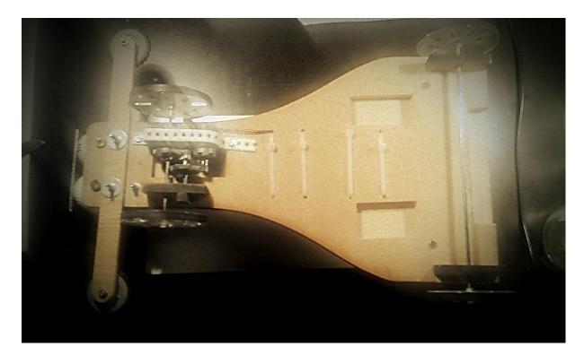
Every axle (3) visible on the picture is provided with 2 bearing located in the wooden parts. This was actually a tricky part to produce because the bearings can't fall out and they had to stand straight. In the picture below the different parts provided with a bearing can be seen.
