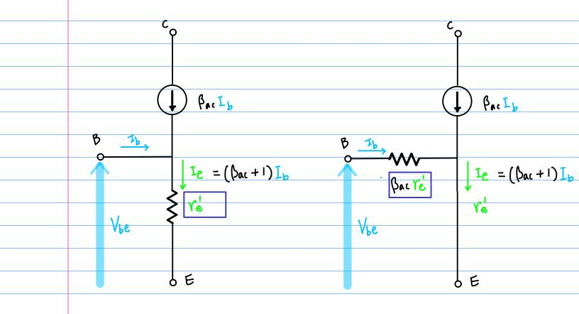
$$V_{be} = I_{e} r_{e}' = (\beta \alpha c + 1) I_{b} r_{e}'$$
