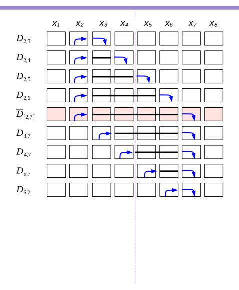
$\overline{D}_{[2,7]}$  = the maximum delay of carry signals  $\leq D$  generated in the i-th group and terminated in the j-th group such that  $2 \leq i, j \leq 7$
