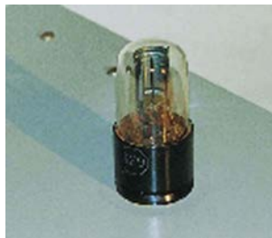
Figure 29.7 The photoelectric effect can be observed by allowing light to fall on the metal plate in this evacuated tube. Electrons ejected by the light are collected on the collector wire and measured as a current. A retarding voltage between the collector wire and plate can then be adjusted so as to determine the energy of the ejected electrons. For example, if it is sufficiently negative, no electrons will reach the wire. (credit: P.P. Urone)
