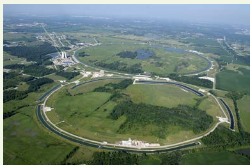
Figure 28.23 The Fermi National Accelerator Laboratory, near Batavia, Illinois, was a subatomic particle collider that accelerated protons and antiprotons to attain energies up to 1 Tev (a trillion electronvolts). The circular ponds near the rings were built to dissipate waste heat. This accelerator was shut down in September 2011. (credit: Fermilab, Reidar Hahn)
