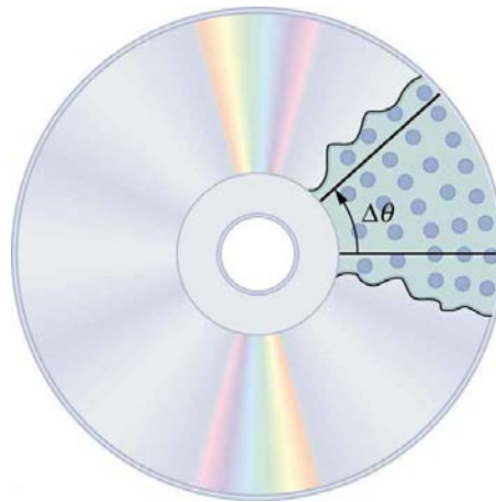
Figure 6.2 All points on a CD travel in circular arcs. The pits along a line from the center to the edge all move through the same angle \Delta\theta in a time \Delta t .
