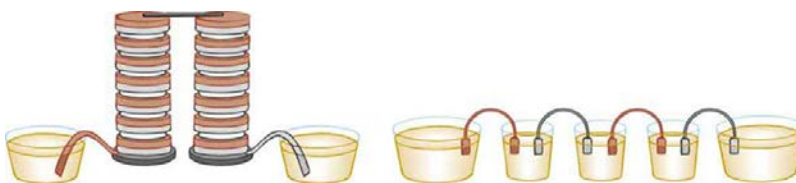
Figure 21.16 Batteries are multiple connections of individual cells, as shown in this modern rendition of an old print. Single cells, such as AA or C cells, are commonly called batteries, although this is technically incorrect.
