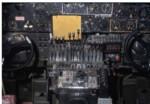
Figure 31.2 The dials of this World War II aircraft glow in the dark, because they are painted with radium-doped phosphorescent paint. It is a poignant reminder of the dual nature of radiation. Although radium paint dials are conveniently visible day and night, they emit radon, a radioactive gas that is hazardous and is not directly sensed. (credit: U.S. Air Force Photo)
