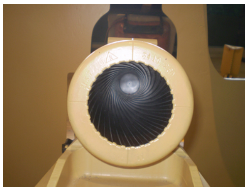
Figure 10.36 The image shows a view down the barrel of a cannon, emphasizing its rifling. Rifling in the barrel of a canon causes the projectile to spin just as is the case for rifles (hence the name for the grooves in the barrel). (credit: Elsie esq., Flickr)
