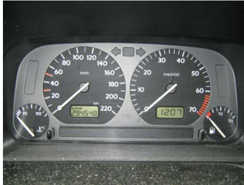
Figure 21.26 The fuel and temperature gauges (far right and far left, respectively) in this 1996 Volkswagen are voltmeters that register the voltage output of “sender” units, which are hopefully proportional to the amount of gasoline in the tank and the engine temperature. (credit: Christian Giersing)
