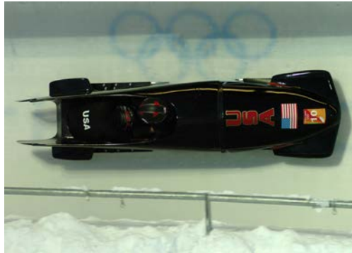
Figure 5.8 From racing cars to bobsled racers, aerodynamic shaping is crucial to achieving top speeds. Bobsleds are designed for speed. They are shaped like a bullet with tapered fins. (credit: U.S. Army, via Wikimedia Commons)
