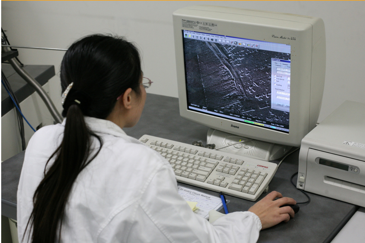
Figure 26.1 A scientist examines minute details on the surface of a disk drive at a magnification of 100,000 times. The image was produced using an electron microscope. (credit: Robert Scoble)
