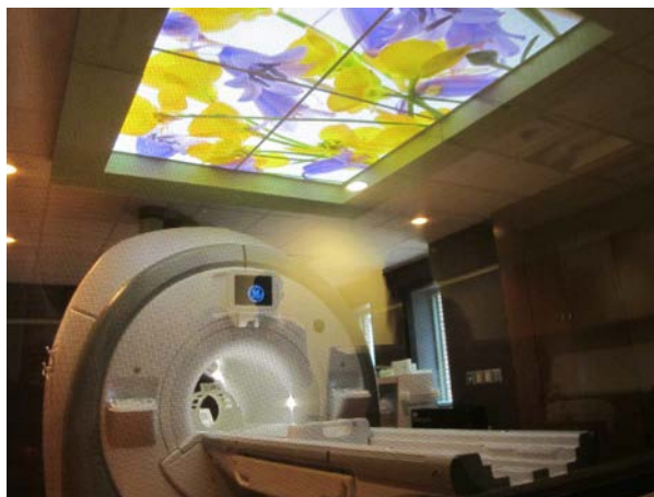
Figure 22.9 Instrument for magnetic resonance imaging (MRI). The device uses a superconducting cylindrical coil for the main magnetic field. The patient goes into this "tunnel" on the gurney. (credit: Bill McChesney, Flickr)
