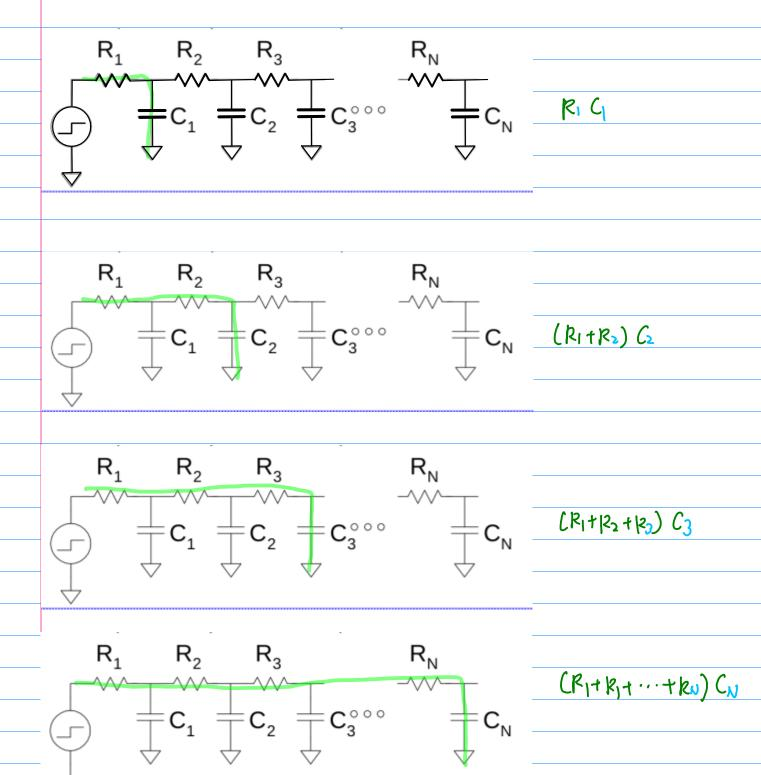
$$t_{pd} = R_1 C_1 + (R_1 + R_2) C_2 + \dots + (R_1 + R_2 + \dots + R_N) C_N$$
