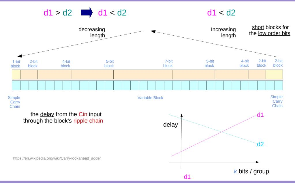
We use a block length <u>from low order</u> to <u>high order cells</u> of 2, 2, 4, 5, 7, 5, 4, 2, 1 for a normal 32 bit structure
