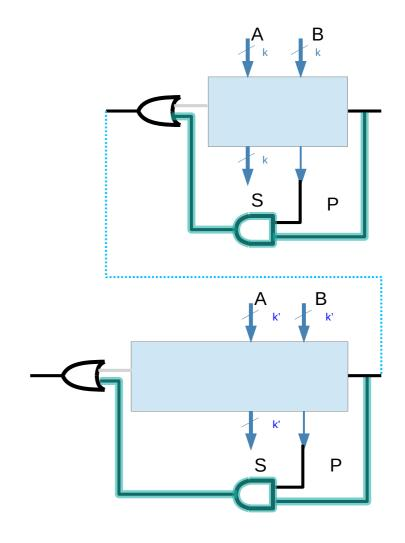
The longest path length through the carry skip block is potentially much shorter than the path from carry-in to carry-out through a ripple carry block.
