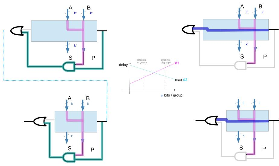
All carries propagated more quickly by varying the block sizes Accordingly the initial blocks of the adder are made smaller, so as to quickly detect carry generates that must be propagated
