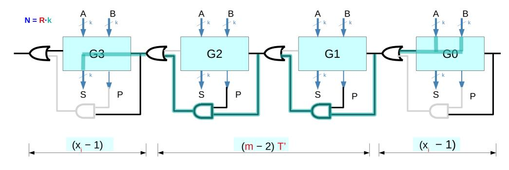
$\Delta_{rca} = 1$  ripple delay over a bit
