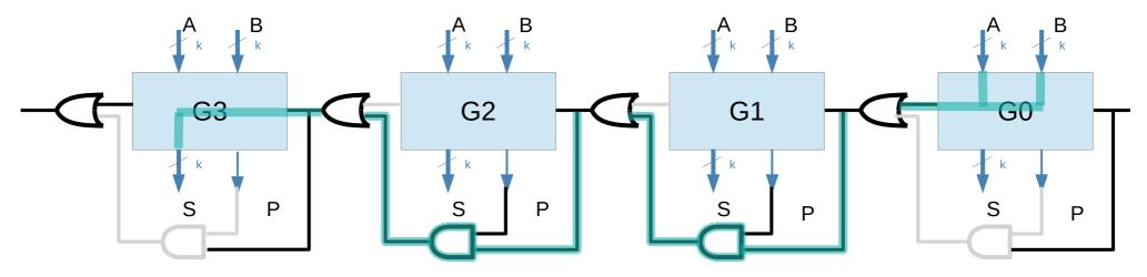
however, <u>unlike</u> the <u>carry select</u> structure, the <u>variable block</u> adder must also worry about the <u>delay</u> from the <u>Cin</u> input through the block's <u>ripple chain</u>
