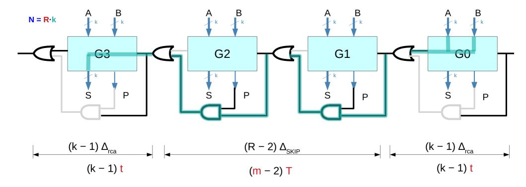
t denote the time required for a carry signal to ripple across a bit
