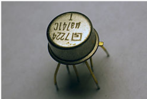
A \mu A741 integrated circuit, one of the most successful operational amplifiers.
