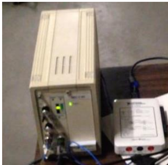
Figure 38 On the left amplifier, on the right the DAQ
