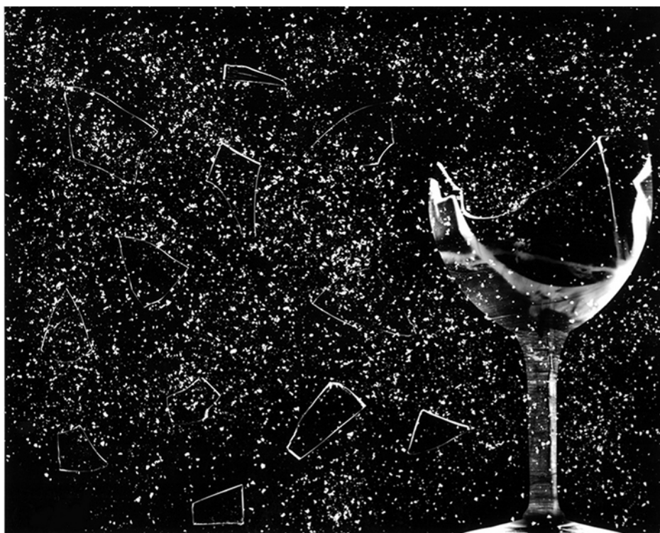
Figure 17.2 This glass has been shattered by a high-intensity sound wave of the same frequency as the resonant frequency of the glass. (credit: “||read||”/Flickr)
