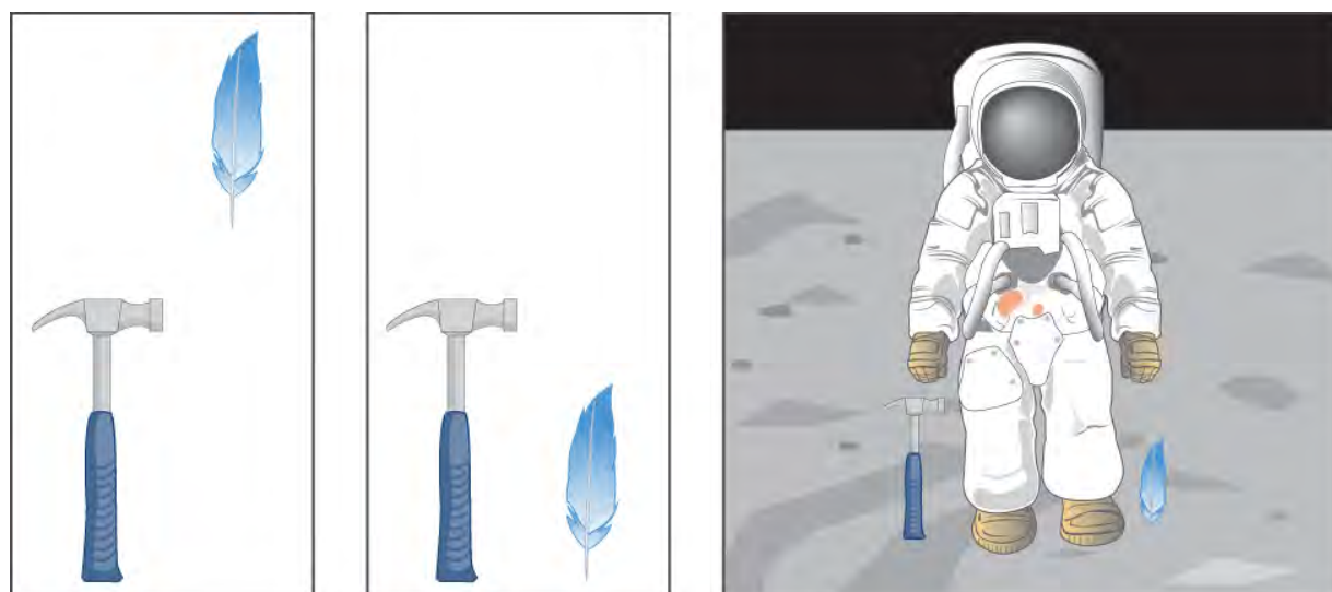
Figure 3.26 In air In a vacuum In a vacuum (the hard way) A hammer and a feather fall with the same constant acceleration if air resistance is negligible. This is a general characteristic of gravity not unique to Earth, as astronaut David R. Scott demonstrated in 1971 on the Moon, where the acceleration from gravity is only 1.67 \text{ m/s}^2 and there is no atmosphere.
