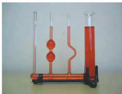
Figure 14.9 If a fluid can flow freely between parts of a container, it rises to the same height in each part. In the container pictured, the pressure at the bottom of each column is the same; if it were not the same, the fluid would flow until the pressures became equal.
