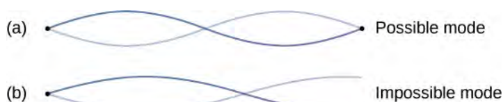
Figure 16.31 (a) The figure represents the second mode of the string that satisfies the boundary conditions of a node at each end of the string. (b) This figure could not possibly be a normal mode on the string because it does not satisfy the boundary conditions. There is a node on one end, but an antinode on the other.
