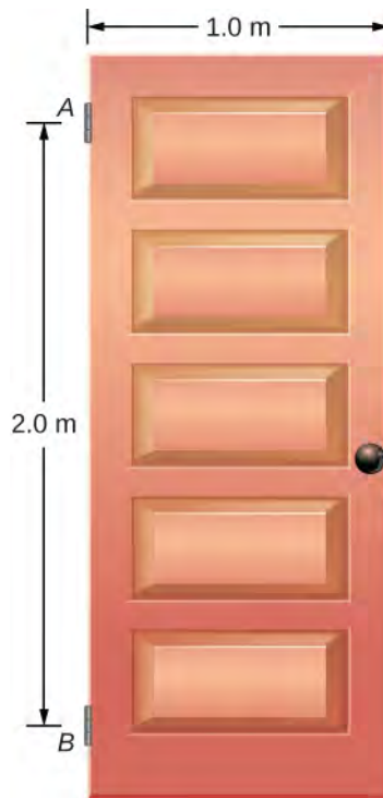
Figure 12.16 A 400-N swinging vertical door is supported by two hinges attached at points A and B.
