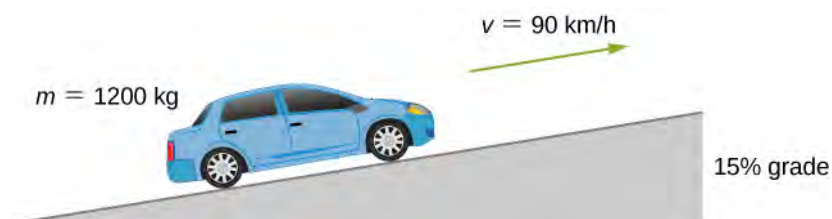
Figure 7.15 We want to calculate the power needed to move a car up a hill at constant speed.
