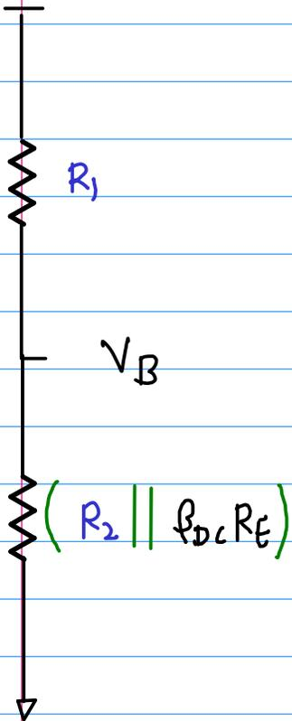
$$V_B = \frac{(R_2 \parallel \beta_{DC} R_E)}{R_1 + (R_2 \parallel \beta_{DC} R_E)} \cdot V_{CC}$$
