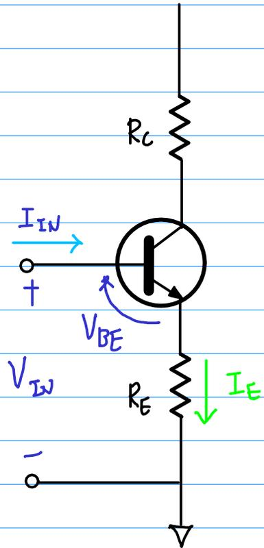
$$\begin{aligned} V_{IN} &= V_{BE} + I_E R_E \\ &\approx I_E R_E \\ &\approx \beta_{DC} I_B R_E \end{aligned}$$
