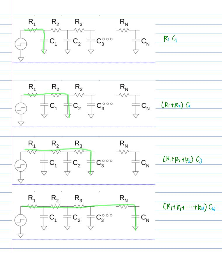
$$t_{pd} = R_1 C_1 + (R_1 + R_2) C_2 + \dots + (R_1 + R_2 + \dots + R_N) C_N$$
