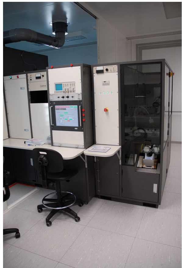
An ion implantation system at LAAS technological facility in Toulouse, France.
