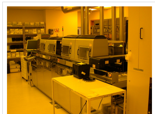
The wafer track portion of an aligner that uses 365 nm ultraviolet light
