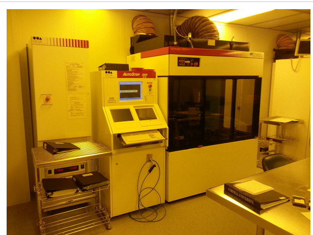
An i-line stepper at Cornell NanoScale Science and Technology Facility. (Photo taken under inactinic light.)
