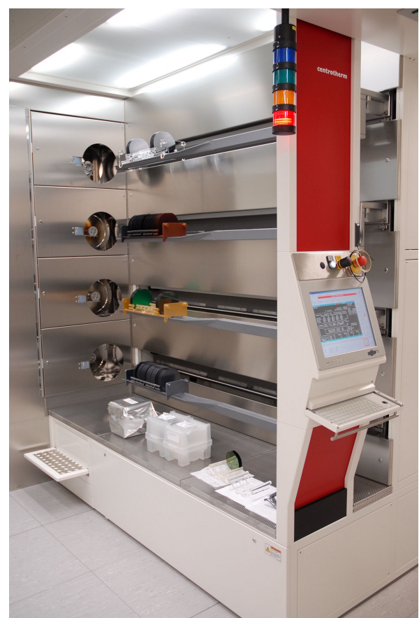
Furnaces used for diffusion and thermal oxidation at LAAS technological facility in Toulouse, France.
