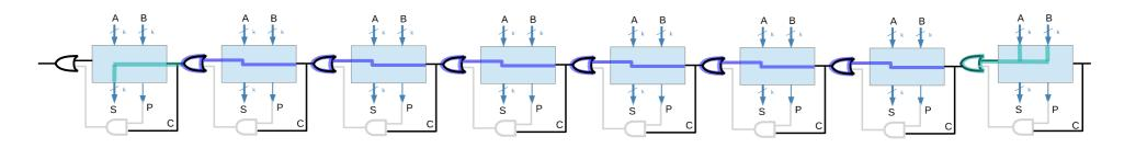
Delay d3 from A, B, Ci to Co – ripple carry delay
