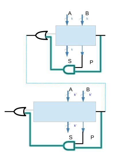
The longest path length through the carry skip block is potentially much <u>shorter</u> than the path from carry-in to carry-out through a ripple carry block.
