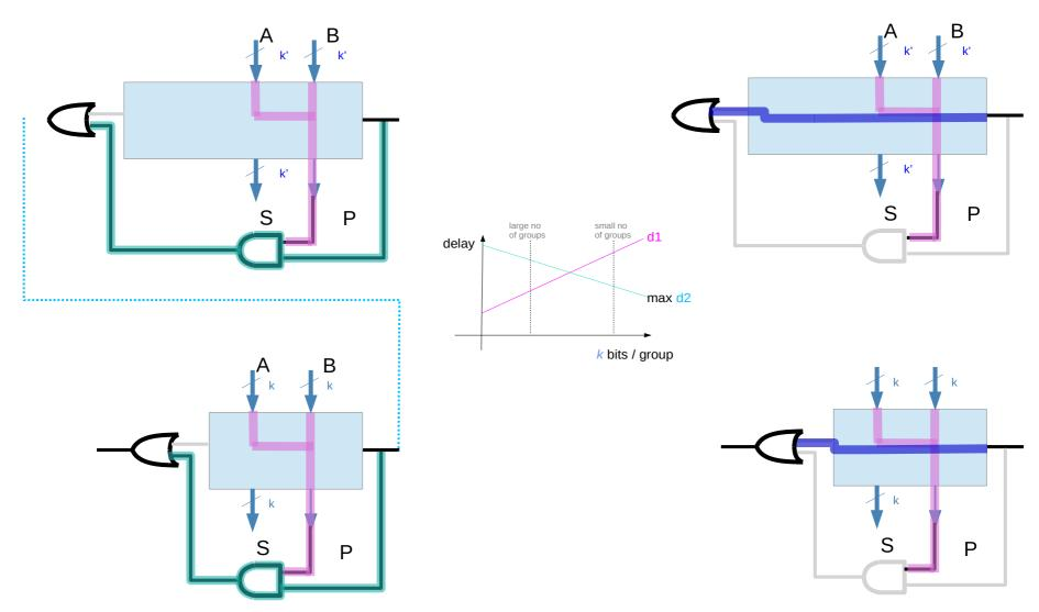
All carries propagated more quickly by varying the block sizes Accordingly the initial blocks of the adder are made smaller, so as to quickly detect carry generates that must be propagated
