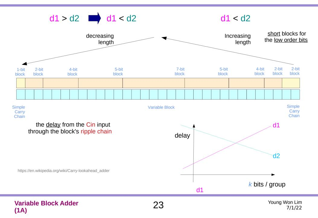
We use a block length <u>from low order</u> to <u>high order cells</u> of 2, 2, 4, 5, 7, 5, 4, 2, 1 for a normal 32 bit structure
