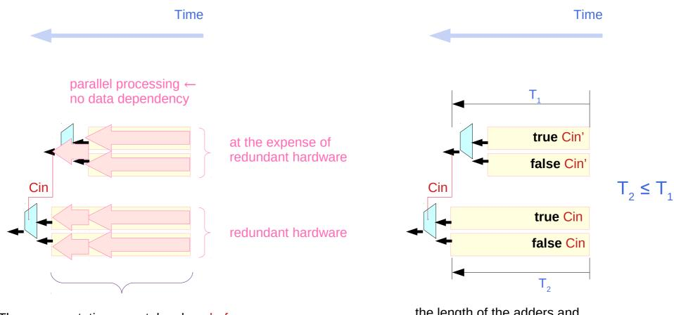
These computations can take place <u>before</u> the completion of the previous columns, since they do <u>not</u> depend on the <u>actual value</u> of the Cin signal the length of the adders and the breakpoint are carefully chosen such that the **adders** finish computations just as their Cin become available
