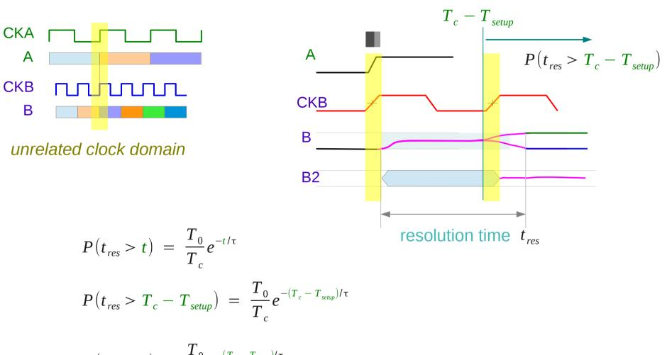
$$P(failure) = \frac{T_0}{T_c} e^{-(T_c - T_{setup})/\tau}$$
