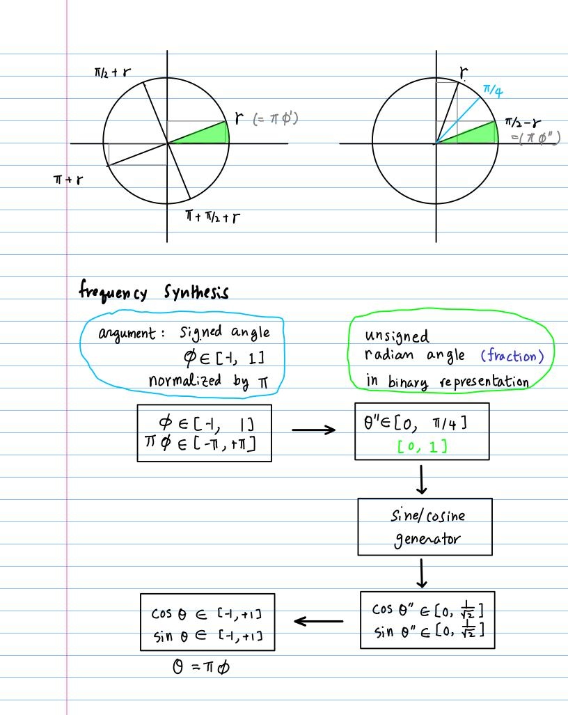
(2)  $\phi \in [-1, 1]$  $\pi \phi \in [-\pi, +\pi]$ θ"∈[0, π/4] [0,1] Sine/ cosine (3) generator (4) $\cos \Theta'' \in [0, \frac{1}{\sqrt{2}}]$ COS 0 E [-1,+1] sin 0" ∈ [0, 長] Sin 0 € [-1,+1]  $\theta = \pi \phi$  $\phi \in [1, 1]$ (1) a phase accumulator 0,1] (2) a radian converter 3 a sine/cosine generator sin O", cos O" @ an output stage Sin Q, cos Q
