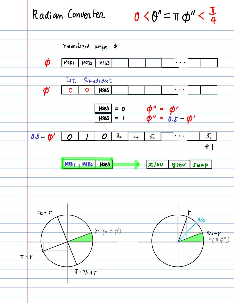
Angle Recoding  $|MSB_1| |MSB_2| |MSB_3| \implies 0 < \theta'' < 1 \implies recoding \{r_k\}$  $\sum_{k=1}^{N} b_k \cdot 2^{-k} = \phi_0 + \sum_{k=2}^{N+1} r_k \cdot 2^{-k}$  $b_k \in \{0, 1\}$   $\Gamma_k \in \{-1, +1\}$  $\varphi_{\circ}$  depends only on bit widith N for fixed N,  $\phi_0 = \frac{1}{2} - \frac{1}{2^{N+1}}$  is a constant
