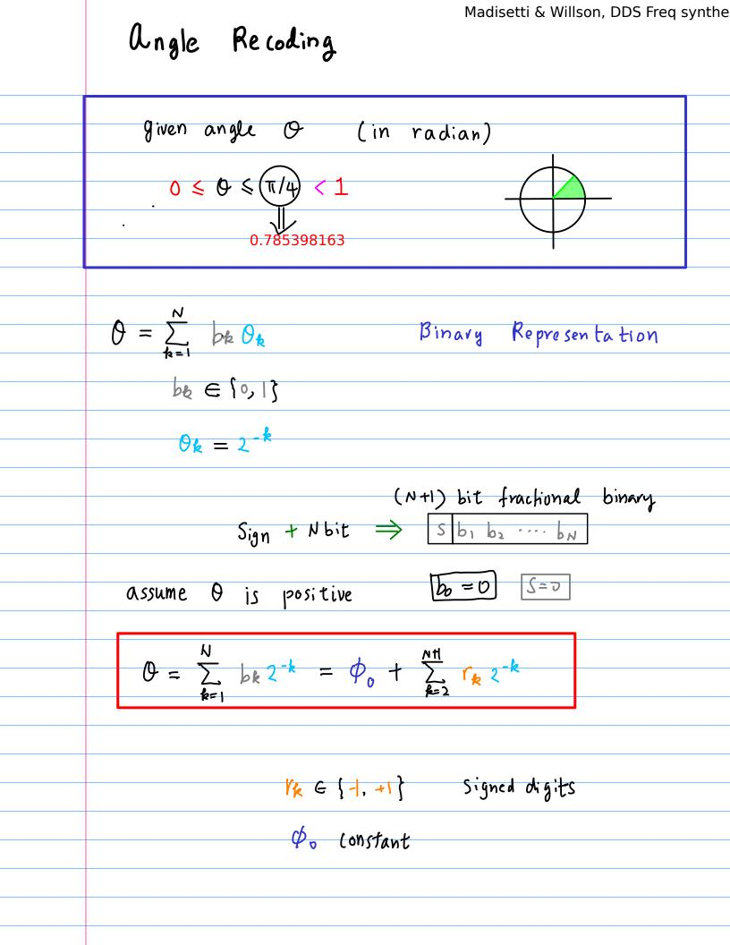
+ subrotation by 2-k 2 equal half rotations by 2<sup>-k+</sup> (FF) () Subrotation 2 equal opposite half rotations by 12-k-1 HA DA Binary Representation bk = 1 : rotation by 2-k be = 0 ; Zero rotation fixed Pos  $2^{-k-1}$  rotation Pos  $2^{-k-1}$  rotation  $\leftarrow b_k = 1$ Pos  $2^{-k-1}$  rotation Meg  $2^{-k-1}$  rotation  $\leftarrow b_k = 0$ R-th rotation Combining all the fixed rotations → initial fixed votation
