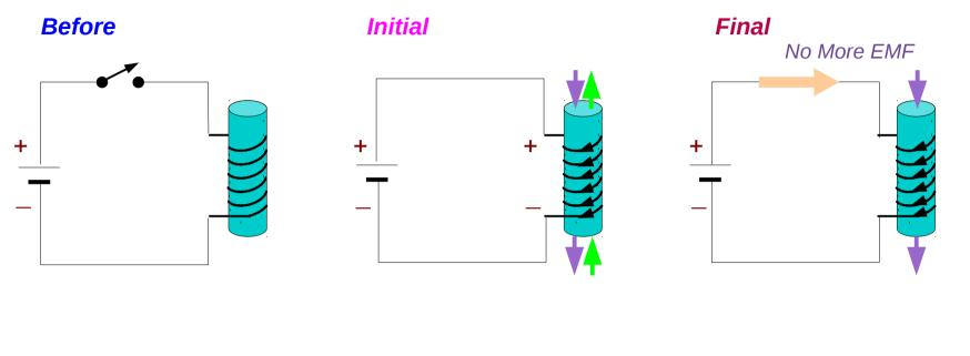
Induced EMF  $v_c(0^-) \neq v_c(0^+)$  voltage jump  $i_c(0^-) = i_c(0^+)$  unyielding current Energy stored in Electric Field
