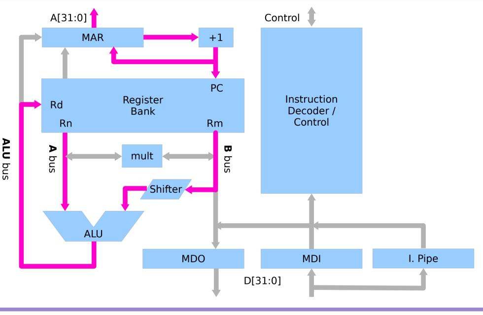
ARM Architecture (2A) Pipelined Architecture
