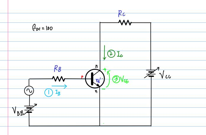
$$\frac{1}{1_{B}} = \frac{V_{BB} - 0.7}{R_{B}}$$
