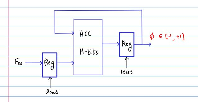
M-bit adder - repeatedly increments the phase of by Fcw at each clock cycle frequency control word at time n,  $\varphi = n \frac{F_{cw}}{2^{M}}$
