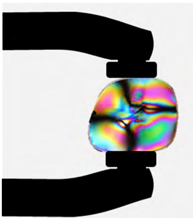
Figure 1.44 Optical stress analysis of a plastic lens placed between crossed polarizers. (credit: "Infopro"/Wikimedia Commons)
