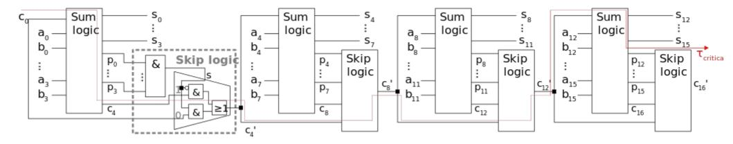
Since the Cin-to-Cout represents the longest path in the ripple-carry-adder, an obvious attempt is to accelerate carry propagation through the adder.
