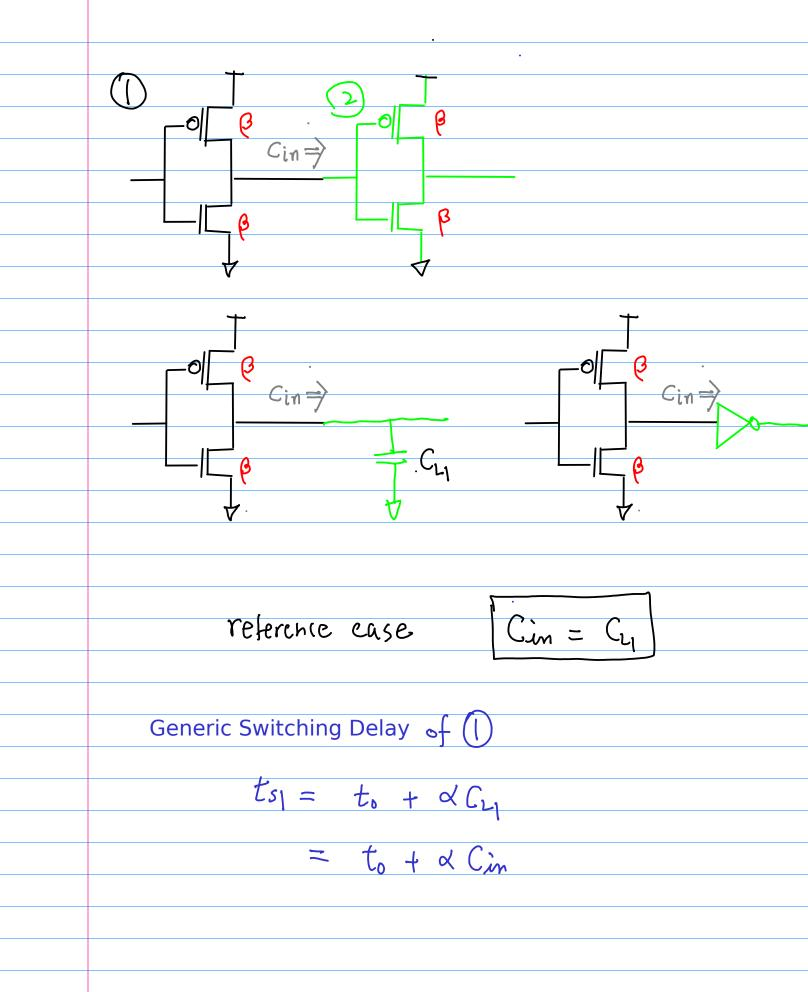
Cin = Can + Cap = Cox (AGn + AGP) Ai gate anea the channel length L assumed Cim = Cox L (Wn + Wp)  $= C_{0x}L(W_n + YW_p)$ =  $C_{0x} \perp W_{p} \cdot (|+r)$ =  $C_{gn}(1+r)$
