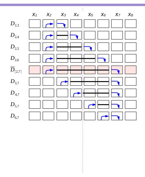
$\overline{D}_{[2,7]}$  = the maximum delay of carry signals  $\leq D$  generated in the i-th group and terminated in the j-th group such that  $2 \leq i$ ,  $i \leq 7$
