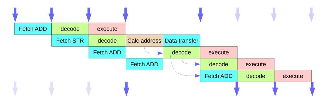
the decode logic is involved in all the <u>decode</u> cycle the <u>address calculation</u> the datapath is involved in all the <u>execute</u> cycle the <u>address calculation</u> the <u>data transfer</u>
