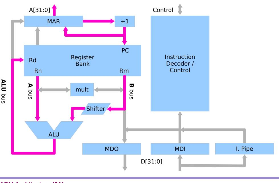
ARM Architecture (2A) Pipelined Architecture
