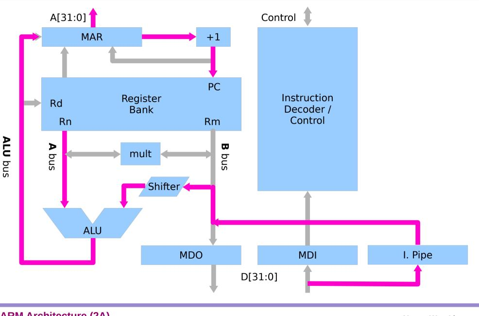
ARM Architecture (2A) Pipelined Architecture
