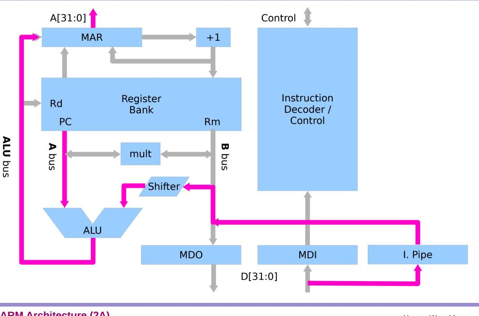
ARM Architecture (2A) Pipelined Architecture
