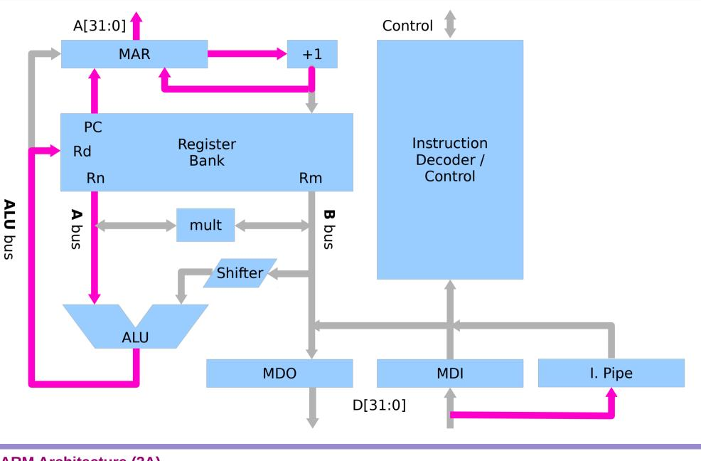
ARM Architecture (2A) Pipelined Architecture
