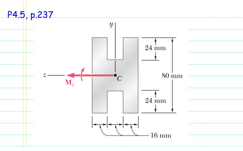
A beam of the cross section shown is extruded from an aluminum alloy for which  $\sigma_Y = 250$  MPa and  $\sigma_U = 450$  MPa. Using a factor of safety of 3.00, determine the largest couple that can be applied to the beam when it is bent about the z axis.
