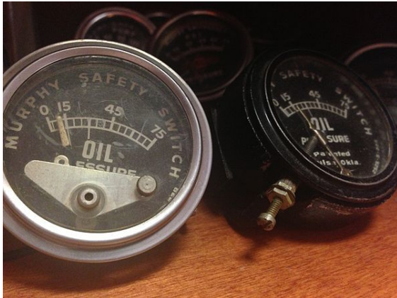
Murphy oil pressure gauges with switches that activate on low pressure
