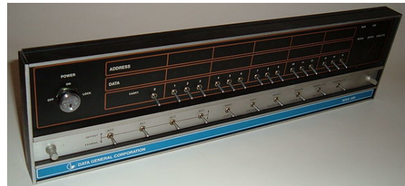
Bank of toggle switches on a Data General Nova minicomputer front panel.
