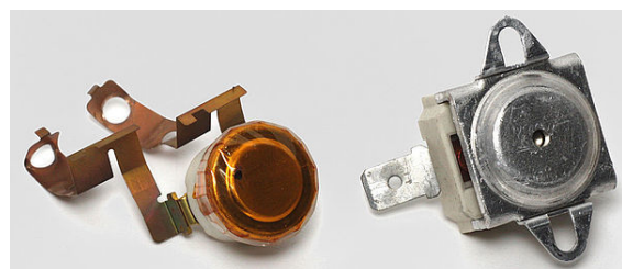
Two thermal switches
