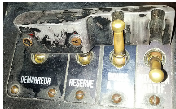
Toggle switches with the shared cover preventing certain forbidden combinations
