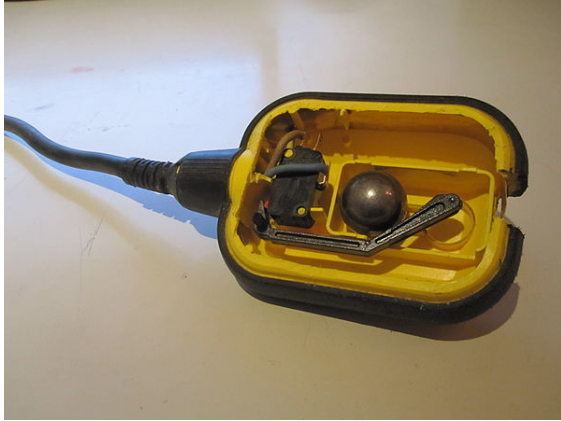
Opened float switch of a dirty water pump
