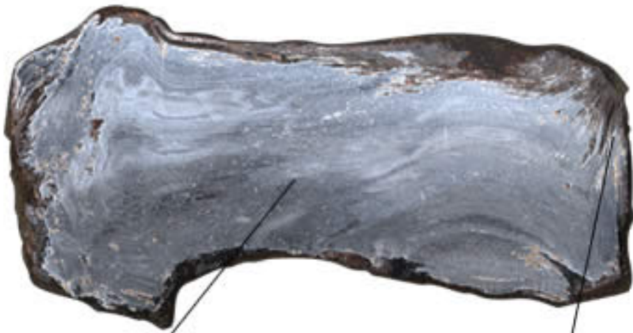
Titanic rivet with a lost head (right)
