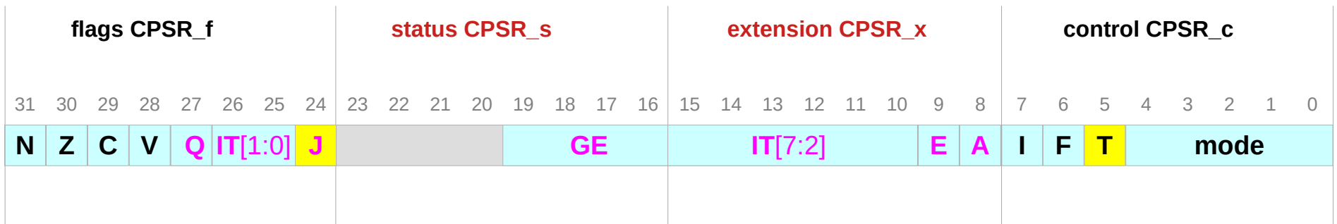
Current Program Status Register (CPSR)
