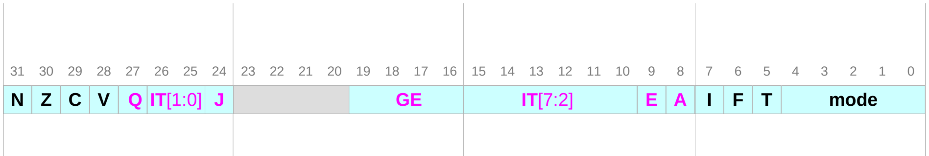
Current Program Status Register (CPSR)
