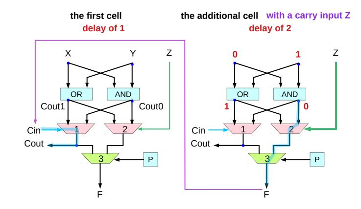
delay of 2(n+1) for an n-bit ripple carry chain with a carry input
