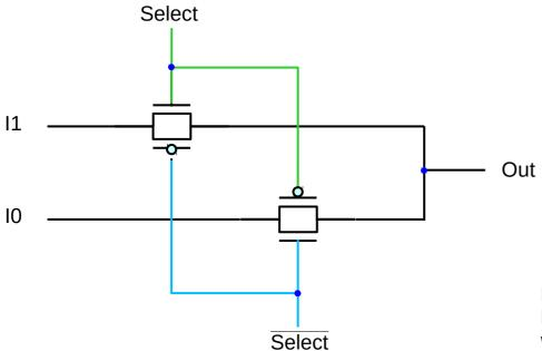
however a mux built with both n-transistor and p-transistor pass gates will operate properly for this case
