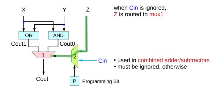
the logic cells - resources to compute a function the exact location of logic cells depends on the user. a user can start or end a carry computation at any place in an fpga. But in many carry computations, the first cell has only 2 inputs, and forcing the carry chain to wait for the arrival of an additional, unnecessary input Z will only needlessly slow down the circuit's computation.
