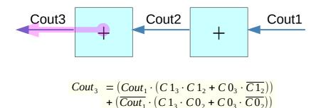
$$\begin{array}{ccc} C \, \mathbf{0}_3 \cdot \overline{C} \, \mathbf{1}_2 \cdot Cout_1 \\ \\ \text{gen} & \overline{\mathbf{prop}} \\ \\ x_3 Y_3 & \overline{x_2} \overline{Y_2} \end{array}$$
