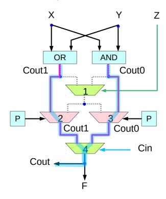
a delay of 2 in the first cell when a carry input is not used
