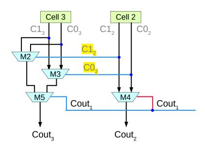
$$(C1_3 C1_2 + C0_3 \overline{C1}_2)Cout_1 + (C1_3 C0_2 + C0_3 \overline{C0}_2)\overline{Cout}_1$$
