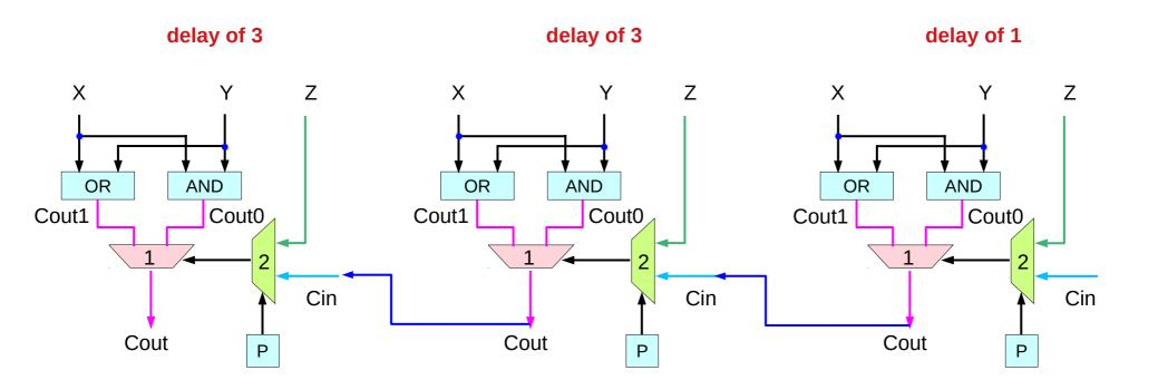
delay of 3n-2 for an n-bit ripple carry chain
