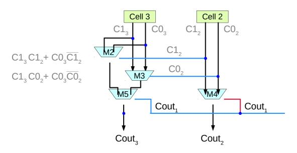
$$(C1_3 C1_2 + C0_3 \overline{C1}_2)Cout_1 + (C1_3 C0_2 + C0_3 \overline{C0}_2)\overline{Cout}_1$$
