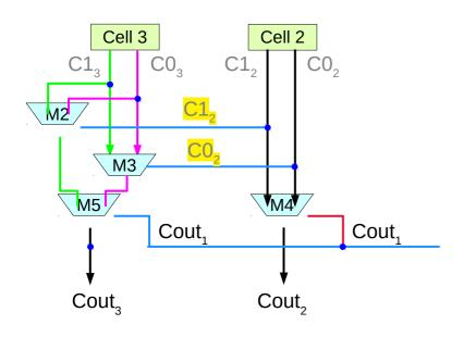
$$(C1_3C1_2 + C0_3\overline{C1}_2)Cout_1 + (C1_3C0_2 + C0_3\overline{C0}_2)\overline{Cout}_1$$
