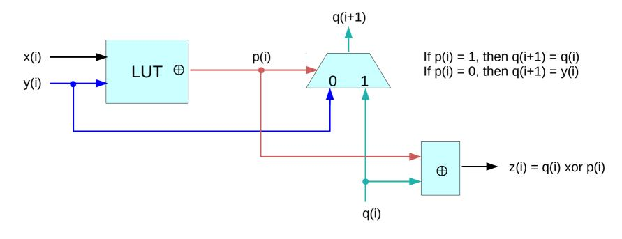
$$\begin{aligned} s_i &= (a_i \oplus b_i) \oplus c_i = p_i \oplus c_i \\ c_{i+1} &= (a_i \cdot b_i) + (a_i \oplus b_i) c_i = \overline{p_i} \cdot g_i + p_i \cdot c_i = \overline{p_i} \cdot a_i + p_i \cdot c_i = \overline{p_i} \cdot b_i + p_i \cdot c_i \end{aligned}$$
