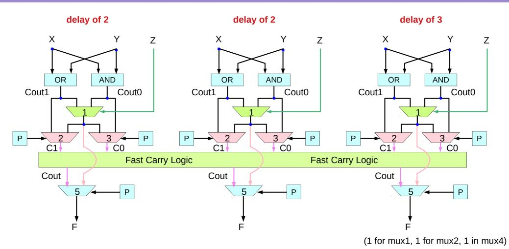
delay of 2n+2 for an n-bit ripple carry chain
