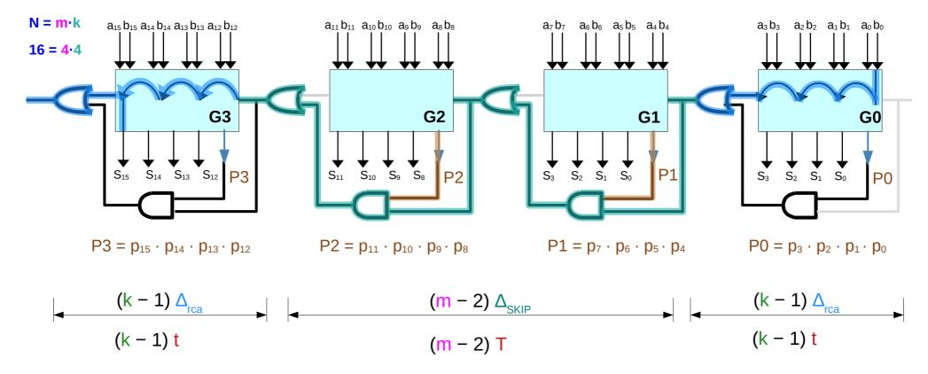
t denote the time required for a carry signal to ripple across a bit
