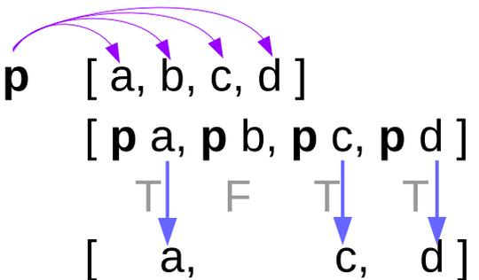
A diagram illustrating the filter function. It shows the input list [a, b, c, d] and the output list [a, c, d]. Above the input list, the predicate 'p' is applied to each element, resulting in a list of booleans [p a, p b, p c, p d]. Below this, the truth values 'T', 'F', 'T', 'T' are shown. Blue arrows point from the 'T' values to the elements 'a', 'c', and 'd' in the output list. A grey 'F' is shown above 'p b' with no arrow pointing to it, indicating it was filtered out.
