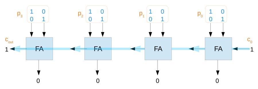
$c_0$  can be propagated to  $c_{out}$  only when s = 1
