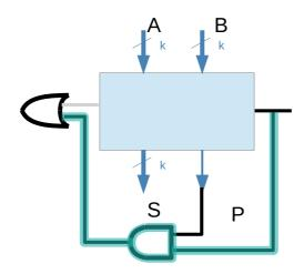
The maximal delay  $\Delta$  of a Carry Skip Adder is encountered when carry is generated in the least-significant bit position,
