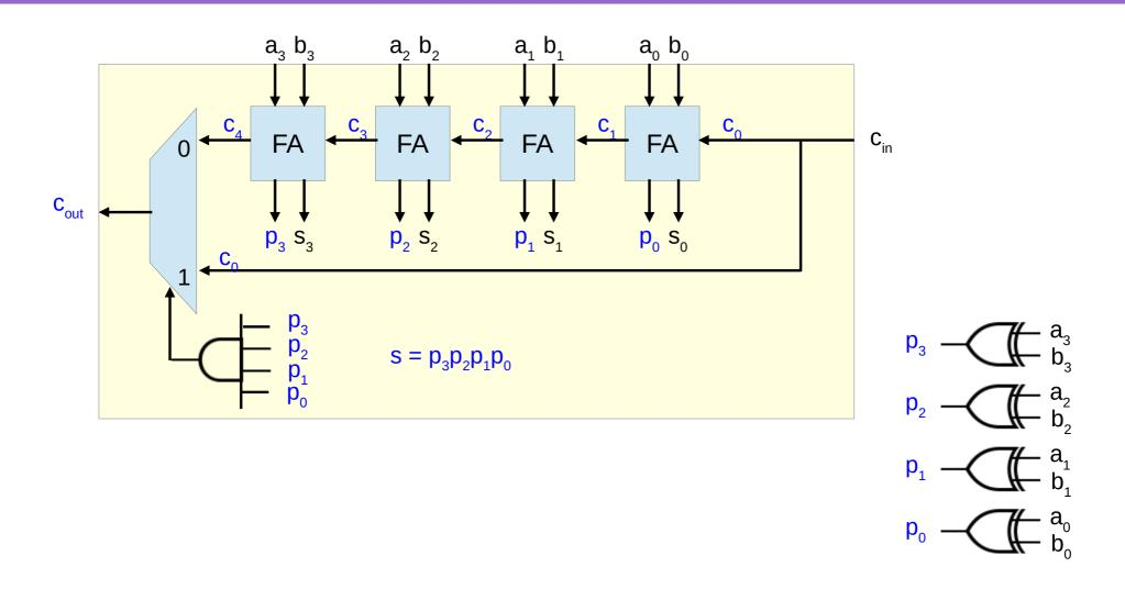
The critical path of a Carry Skip Adder begins at the first full adder, passes through all adders and ends at the sum bit  $s_{n-1}$
