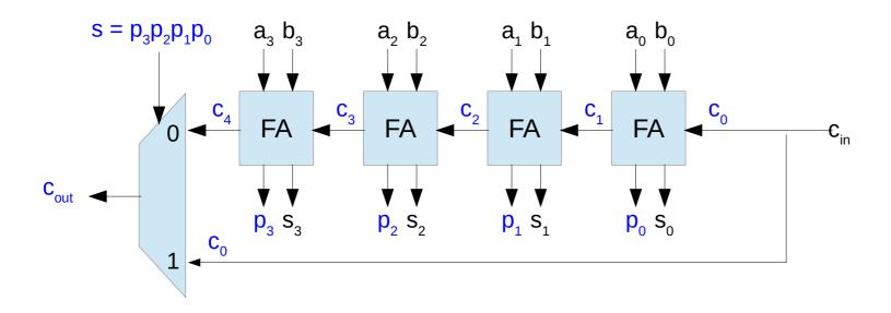
The n-bit-carry-skip adder consists of
